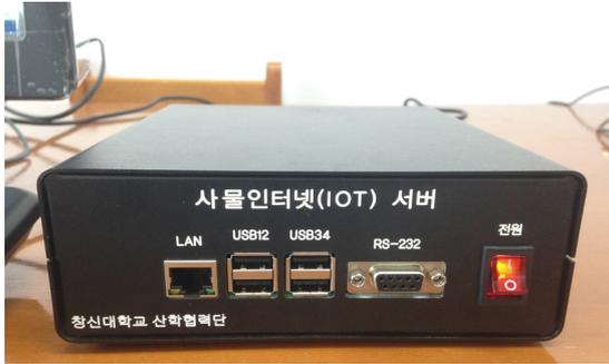
Fig. 6 Implementation of IoT monitoring server
