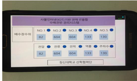
Fig. 8 Distributing board monitoring on Mobile device
