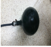
(a) Transducer(ITC-1007)&Transmitting voltage response
