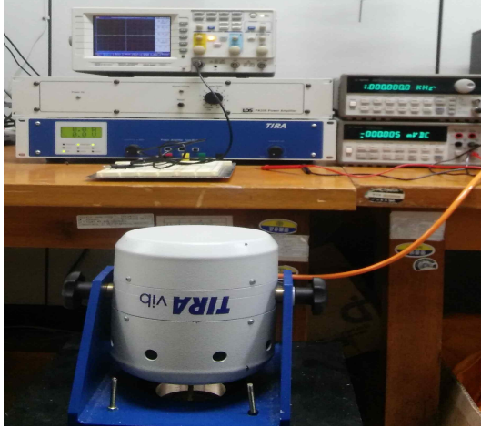
Fig. 8. Measuring setup for applying tensions to the harvester.
