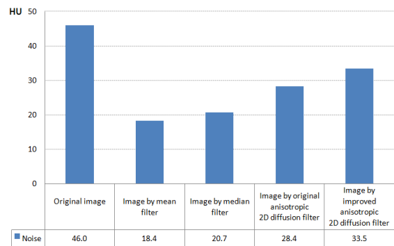
Fig. 6. Evaluation of noise level by original image, image by mean filter, image by median filter and image by anisotropic 2D diffusion based filter.
