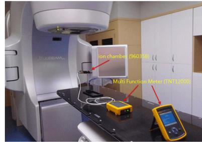
Fig. 1. Measurement of Scattered Rays.
