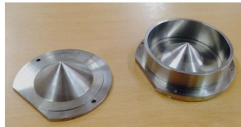
Fig. 2. Flattening Filter.
