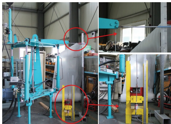
Fig. 8 Experiment for displacement of tip and pendulum
