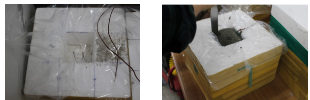
Fig. 2 Test set-up for semi-adiabatic temperature rise test
