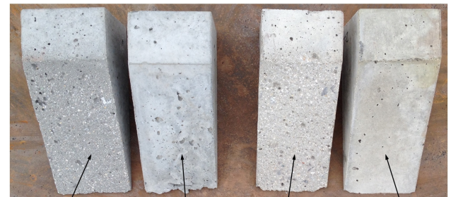
Roughened surface ( f_{ck}=83.8 MPa) No roughness ( f_{ck}=83.8 MPa) Roughened surface ( f_{ck}=31.5 MPa) No roughness ( f_{ck}=31.5 MPa)
