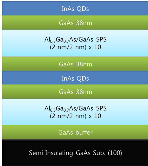
Figure 1. Schematic diagram of InAs quantum dot structure.
