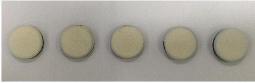
Fig. 1 Delaminate TBC specimen at 1,100°C
