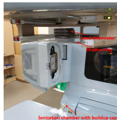
Fig. 2. The experimental setup for half value layer measurement.
