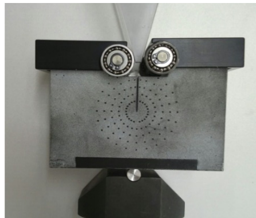
Fig. 1 Static system of WST specimen
