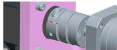
Fig. 11. The motor assembly with coupling
