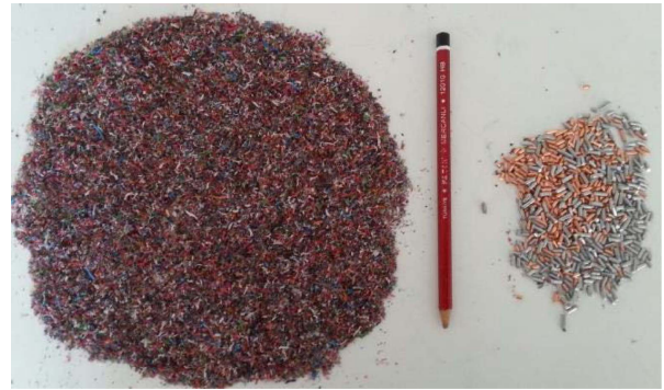
Fig. 15. (Color online) Granule cable waste separation results.
