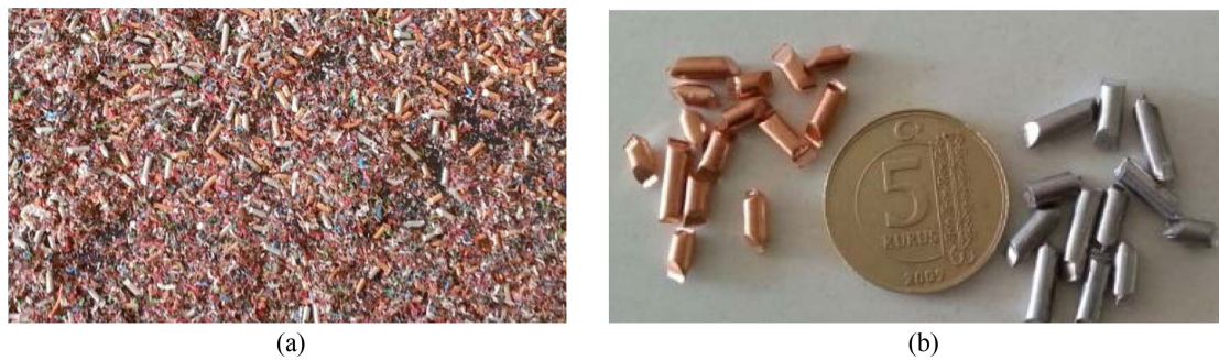
Fig. 6. (Color online) Granule cable waste (a) mixture cable waste with pvc (b) granule cable.
