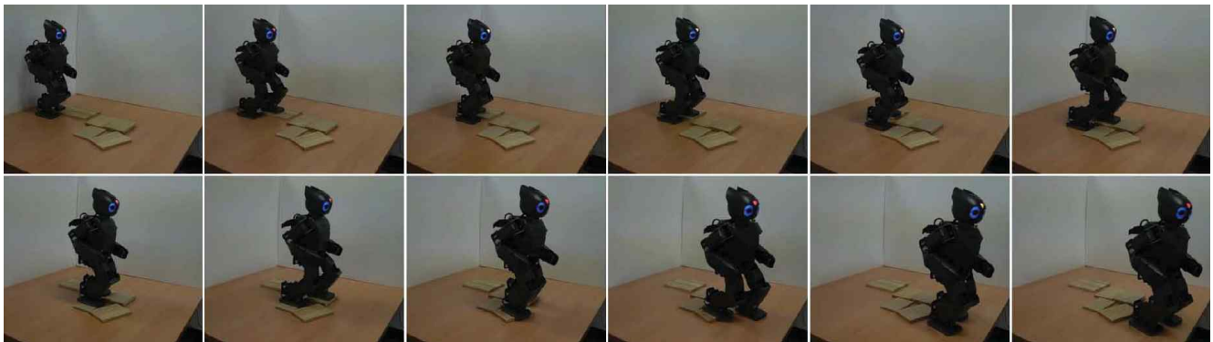
Fig. 5. Snapshots of the walking experiment on unknown uneven terrain (left to right, top to bottom)
