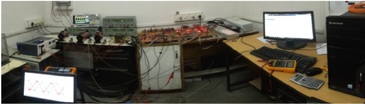
Fig. 16. Experimental setup showing the inverter with load driven by dSPACE 1103
