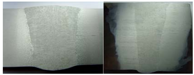
(a) Groove angle 35° (b) Groove angle 20° Fig. 2 EGW cross section at different groove angle
