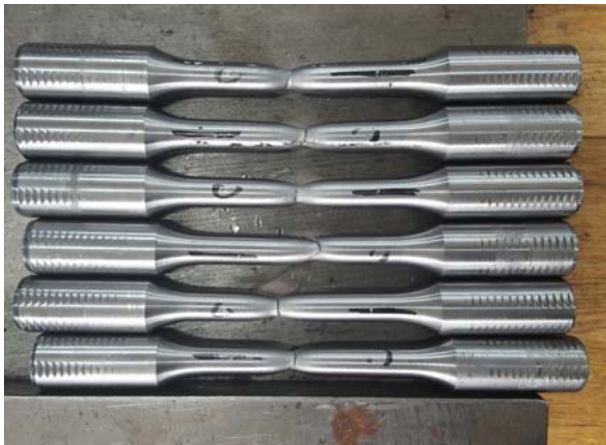
Fig. 16 Test specimen of welding metal after tensile test
