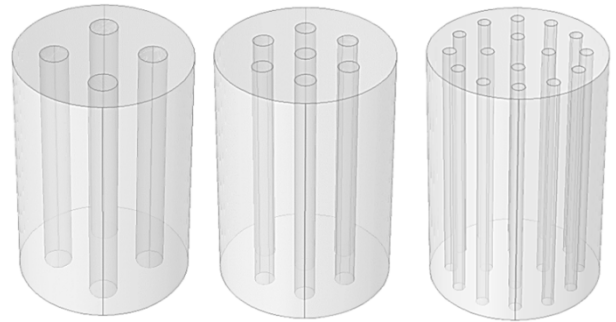
Fig. 7 Computational domain of analysis changed the heat transfer area
