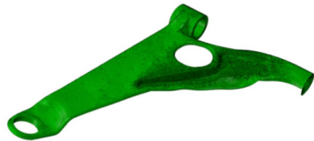
Fig. 5 Finite element shell model of CFRP LCA
