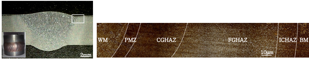
Fig. 2 cross section of the actual weld(a) and Optical microstructures of HAZ(zone denoted as o in (a))
