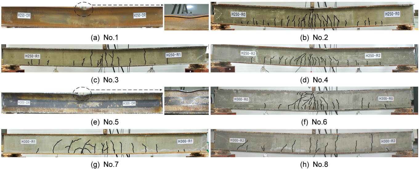
Fig. 8 Crack pattern of bending specimens
