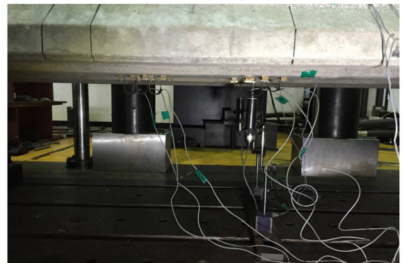
(b) Installed LVDT and crack gauges
