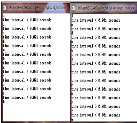
Fig. 6. Time interval measurement: (left) human key input (right) Ducky Script key input
