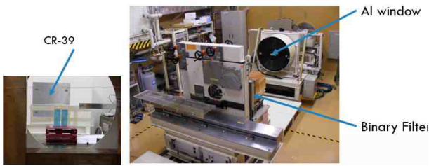
Fig. 1. Experimental setup of CR-39 in HIMAC.
