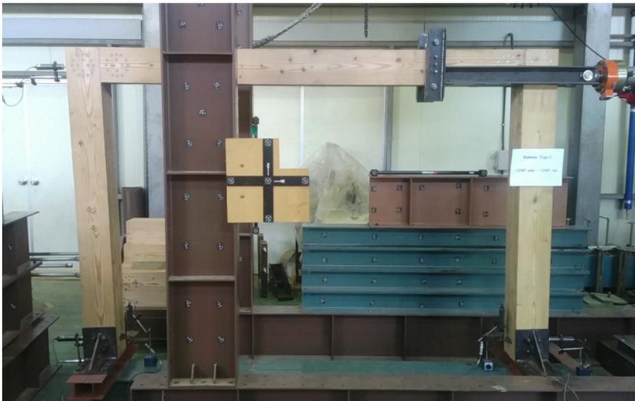
Fig. 3. Test set-up for rahmen structure on laterally cyclic loading.
