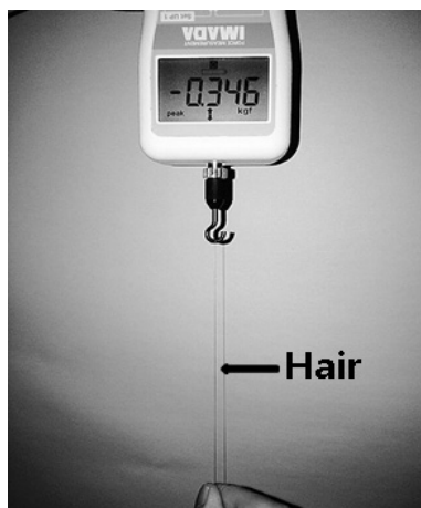
Fig. 1. Tensile test of hair fibers and its results (Son et al., 2015)
