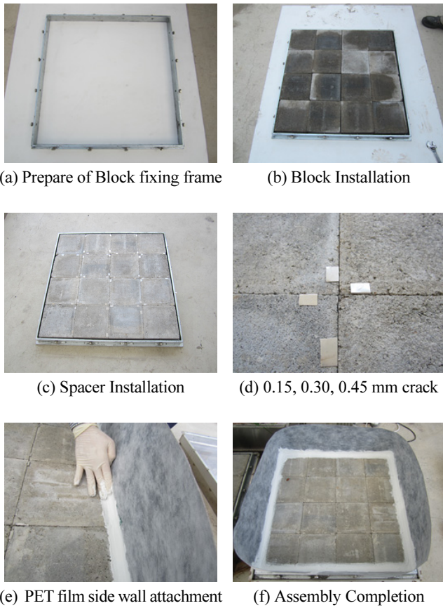
Photo 2 Concrete crack specimen assemble process
