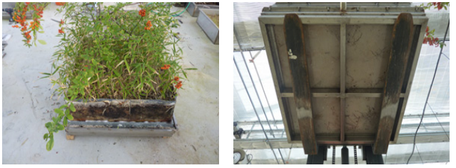
(a) Plant growth state (b) Roots penetration evaluation (12 Months)
