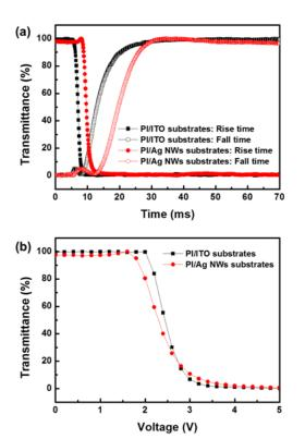
Figure 4. (a) RT curve and (b) V-T curves for the rubbing-aligned LC cells using ITO films and AgNW networks.
