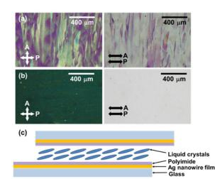
Figure 2. Photomicrographs of the LC cells fabricated by PI/AgNW networks substrates (a) before and (b) after rubbing treatment under the crossed and parallel Nichols (A: analyzer, P: polarizer).
