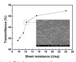
Figure 1. Plot of average transmittance versus sheet-esistance( $R_s$ ) for the Ag NW network films. Inset is a FESEM image of  $R_s \approx 11.3 \, Q/\text{sq}$  Ag NW networks on glass substrate
