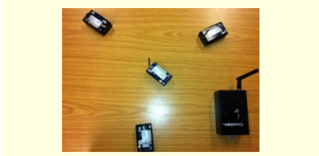
Fig. 5. Capture effect application environment; three senders, one receiver in the middle, and a base station.
