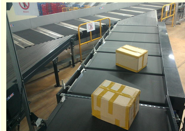
Fig. 12. Picture of sorting system's infeed line used in experiments.
