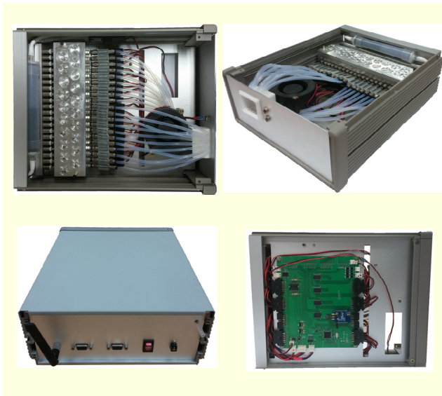
Fig. 3. Developed scent display device.
