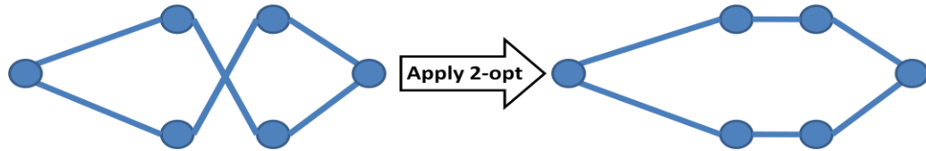
Fig. 1. 2-Opt removes intersecting sub-tours (on the left) and may produce shorter path (on the right)
