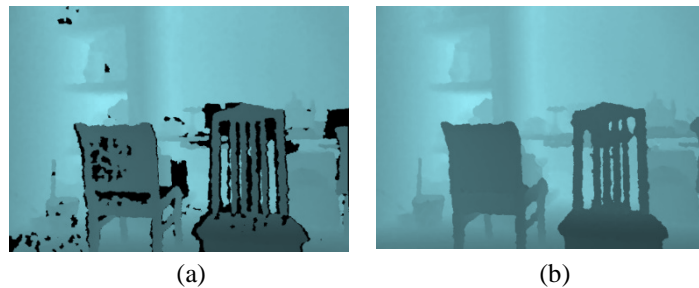
Fig. 2. Depth noise reduction and smoothing: (a) raw depth map, (b) depth map after preprocessing
