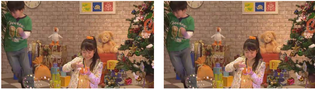
(d) QP = 37. PSNR(left): 30.08 dB; PSNR(right): 29.91 dB; PSNR loss: 0.17 dB.
