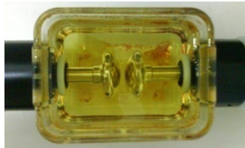
Fig. 1. The electrode used for measuring BDV of oil mixture
