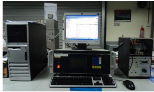
Fig. 4. AVOX ADTR-2k fully automatic Tan delta, dielectric constant and resistivity test set
