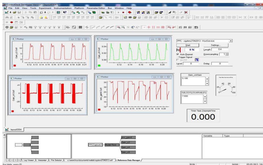
Fig. 9. The real time platform showing the current, voltage, flux linkage waveforms and predicted angle values
