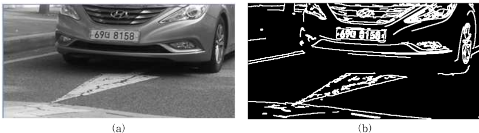
Fig. 2. (a) Reduced gray image, (b) Obtained edges image after applying Gaussian filter.
