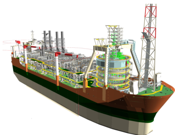
Fig.1 Ship-type turret moored BP Quad 204 FPSO
