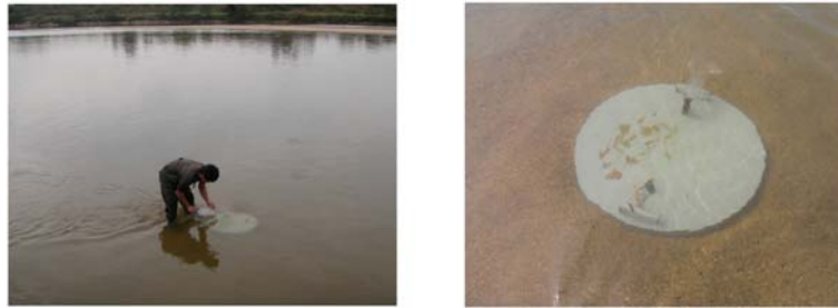
Fig. 3. Illustration of seepage meter plugged into the streambed for study sites.
