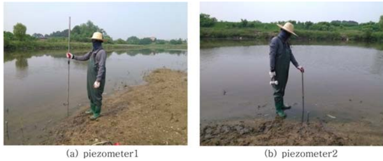
Fig. 4. Piezometers for measurement of hydraulic head in streambed for study sites.
