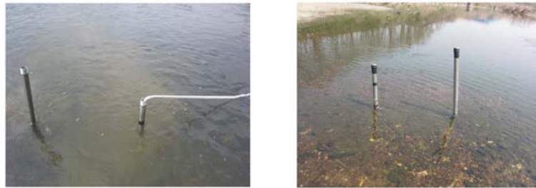
Fig. 5. Illustration of piezometers plugged into the streambed for study sites.
