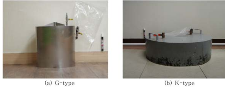
Fig. 2. Seepage meters for water flux measurement through streambed for study sites.
