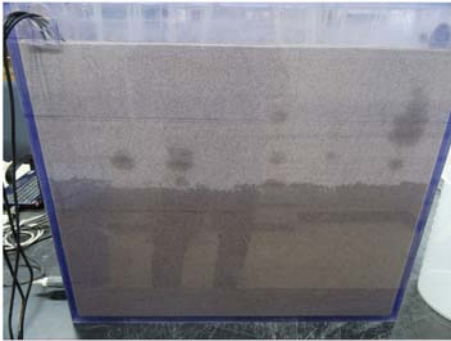
Fig. 10. Saturation process from the bottom of the soil box.
