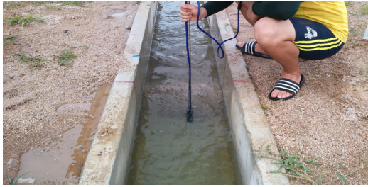
Photo 3 Measurement of flow velocity
