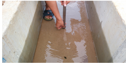
Photo 4 Measurement of sediment height
