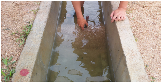
Photo 4 Measurement of sediment height
