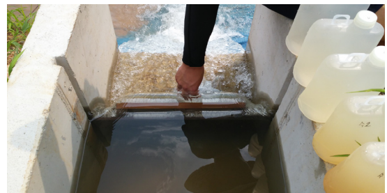
Photo 2 Sampling of suspended sediment concentration
