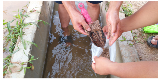
Photo 5 Sampling of soil sediment
