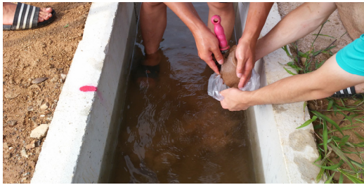
Photo 5 Sampling of soil sediment
