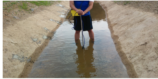
Photo 3 Measurement of flow velocity
