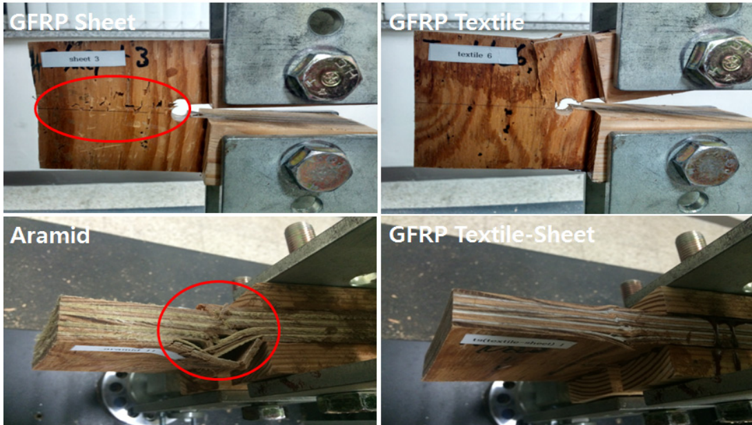
Fig. 6. Failure mode of FRP-reinforced laminated plates.
