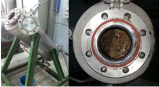
Fig. 1. Digester for steam digestion of wood chips.
