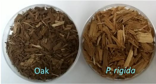
**Fig. 4.** Produced wood-based roughages by digestion for 90 min from oak (left) and *P. rigida* (right).
