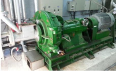
**Fig. 2.** Refiner for wood based roughage manufacture.
