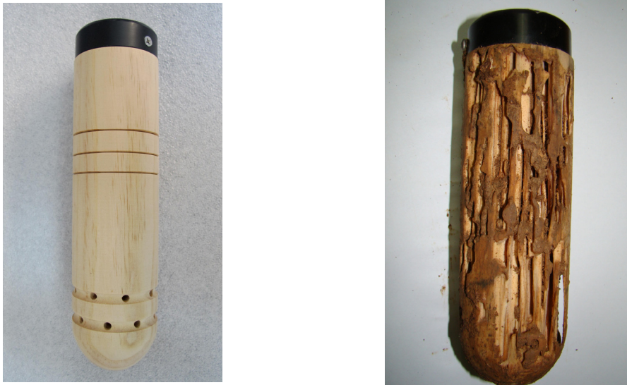
Fig. 3. Termitic damage of wooden station (left: before, right: after feeding).
