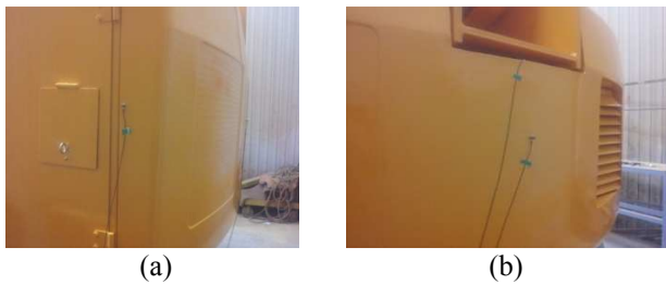
Fig. 5 Vibration measurements during operation; (a) x-axis, (b) y-axis & z-axis
