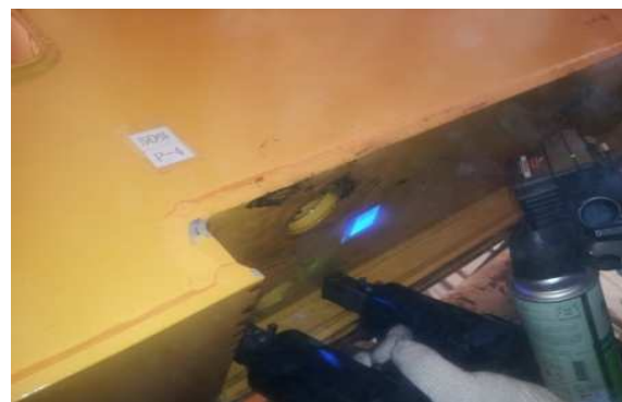
Fig. 12 Non destructive examination after life test
