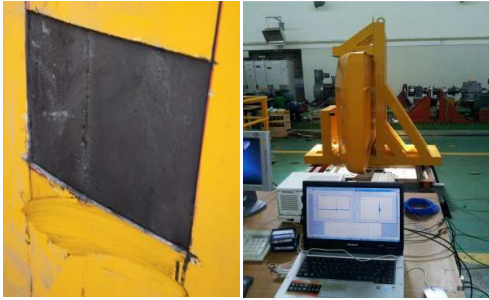
Fig. 9 Counterweight internal photo and impact test equipment
