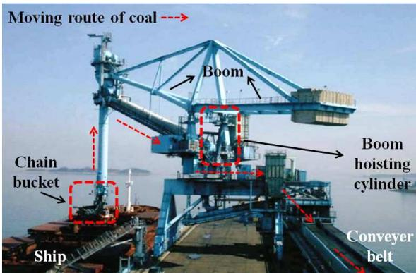
Fig. 1 The coal handling machine
