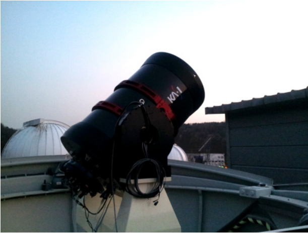
Fig. 2. The optical tube assembly on an Alt-Azi mount at the test-bed of OWL-Net.
