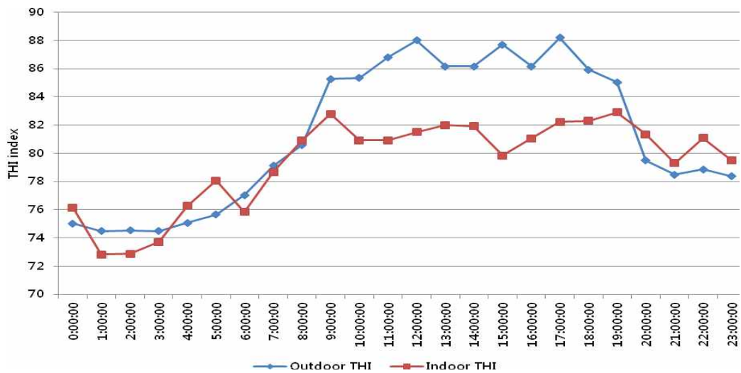
Fig. 3. Changes in hourly temperature-humidity index in cow house with ventilation duct.
