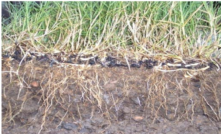
Fig.1. Illustrations of vegetated HPTRM system. The open space of HPTRM allows roots grow through and entwined with the HPTRM to reinforce the plant roots.
