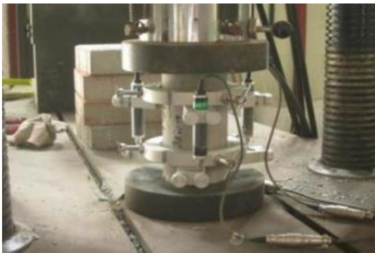
Photo 1. Compressive strength and elasticity modulus test
